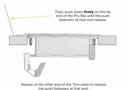
The outlet can then be easily removed.
